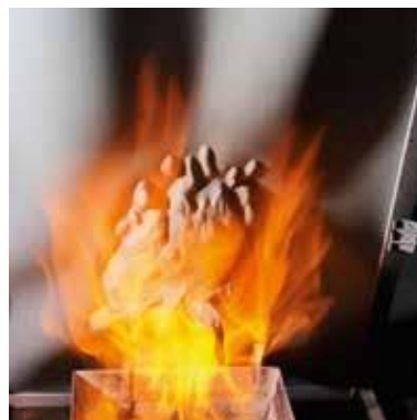
Flame testing of the S-flex product group material according to BS 6853.
