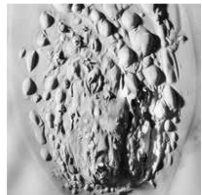
Surface of the S-flex 210 after a 40-minute long smoke density test in compliance with BS 6853 after the flame exposure. The surface resists the flame load, and no cracks in the material are visible.
