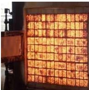
Vertical spread of flame testing of the S-flex product group material according to BS 476 Part 7 Class 1. Heat radiation during the 25 kW / m 2 test.
